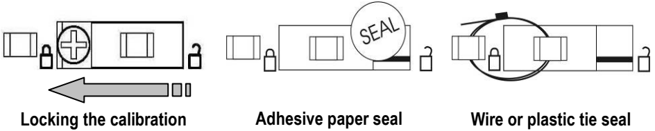
Figure 4-1. Locking and Sealing the Calibration Lock Switch.
